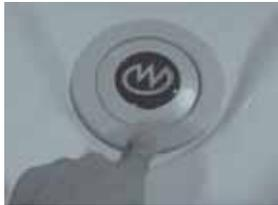
To use the pop-up speaker system, press down on the button located in the corner. This will automatically raise the speaker for use.
