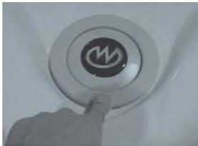
To use the pop-up speaker system, press down on the button located in the corner. This will raise the speaker.
