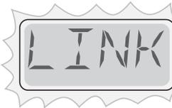
After the startup sequence, LINK will appear if no button has been pressed. Press any button to Link the Panel with the System.
