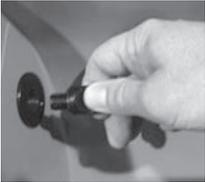
The Momentum 80 and Momentum 50 have an additional air bleed system that helps aid in relieving air locks. There is an air bleed valve located in the filter area of the swim spa portion of the swim spa. When filling the swim spa this should be opened to facilitate relieving any air that may be trapped in the pumps.
