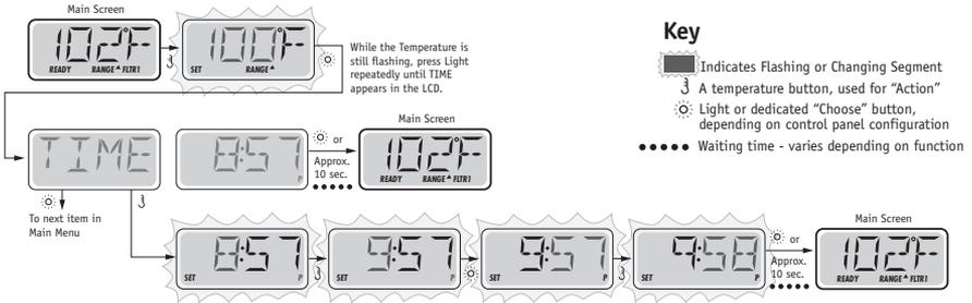
**NOTE:** If power is interrupted to the system, Time-of-Day will need to be reset.
