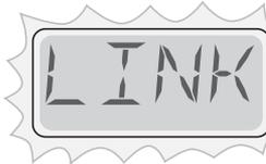
After the startup sequence, LINK will appear if no button has been pressed. Press any button to Link the Panel with the System.
