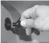
The Momentum 80 and Momentum 50 have an additional air bleed system that helps aid in relieving air locks. There is an air bleed valve located in the filter area of the swim spa portion of the swim spa. When filling the swim spa this should be opened to facilitate relieving any air that may be trapped in the pumps. Make sure that the plug is reinstalled once the spa is running correctly.
