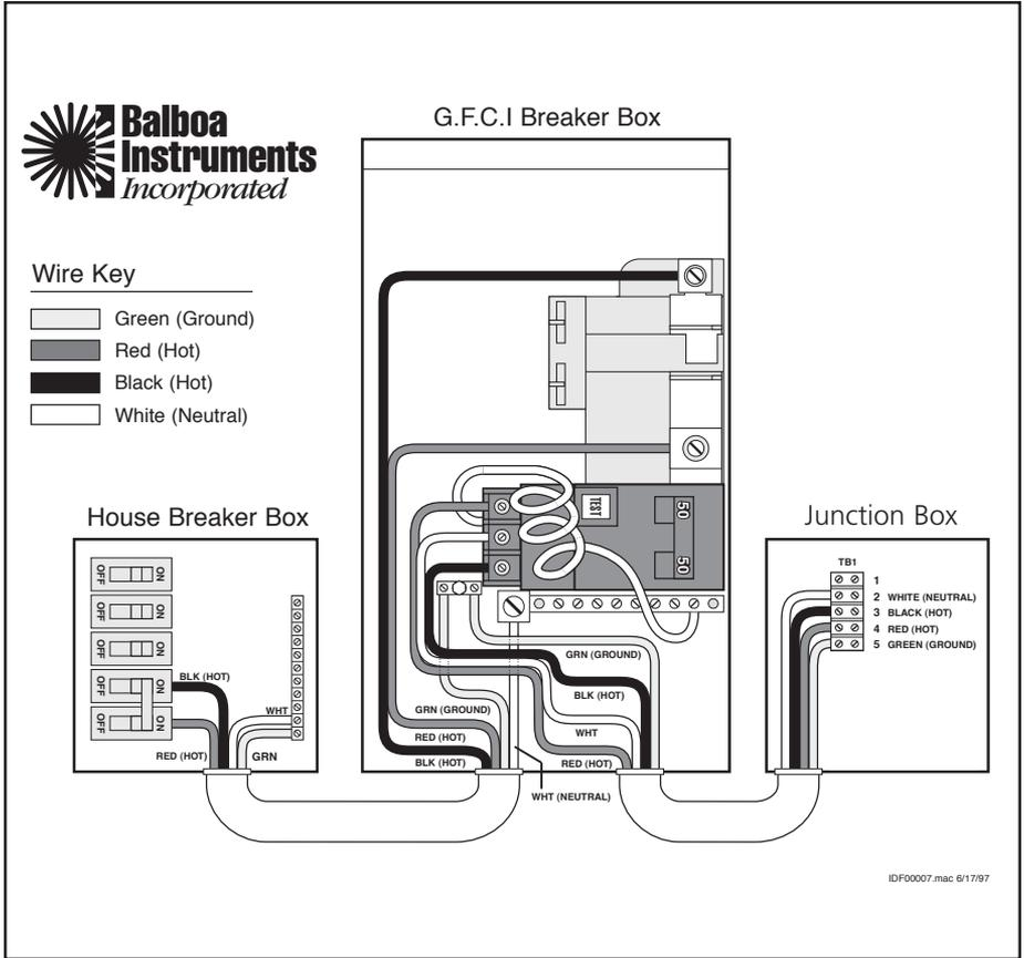
\* Actual wiring of GFCI will vary by manufacturer of GFCI. The GFCI shown is a Square D. Improper wiring of GFCI may result in permanent damage to swim spa system box. Repair / replacement of swim spa system box is not covered under warranty when damage results from improper wiring. Actual wire attachment points on the Spa Control Pack and junction box may vary with different models. Always refer to the wiring diagram inside the Spa Control Pack or junction box for proper connection.
