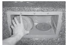
*Install Eco Pur filter on left side.*
