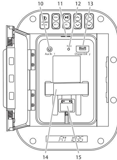
**11. Interior Light:** When the unit is turned on the LEDs will automatically illuminate the interior compartment.
