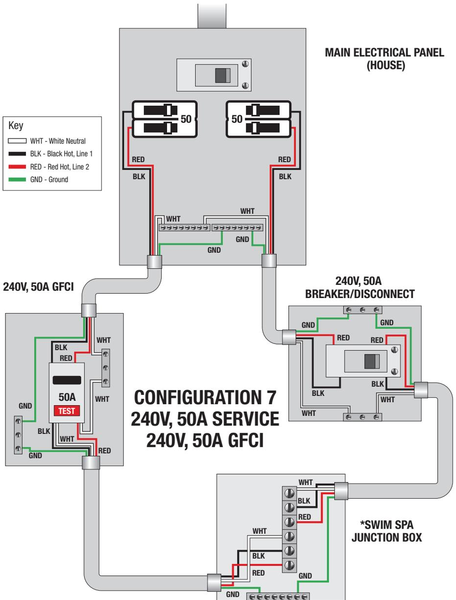
\*Refer to wiring diagram inside swim spa junction box for proper power connection to terminals. The swim spa junction box is located inside swim spa behind the factory installed GFCI. Remove skirt access panel "B" to gain access to swim spa junction box (see Glossary of Swim Spa Terminology).
