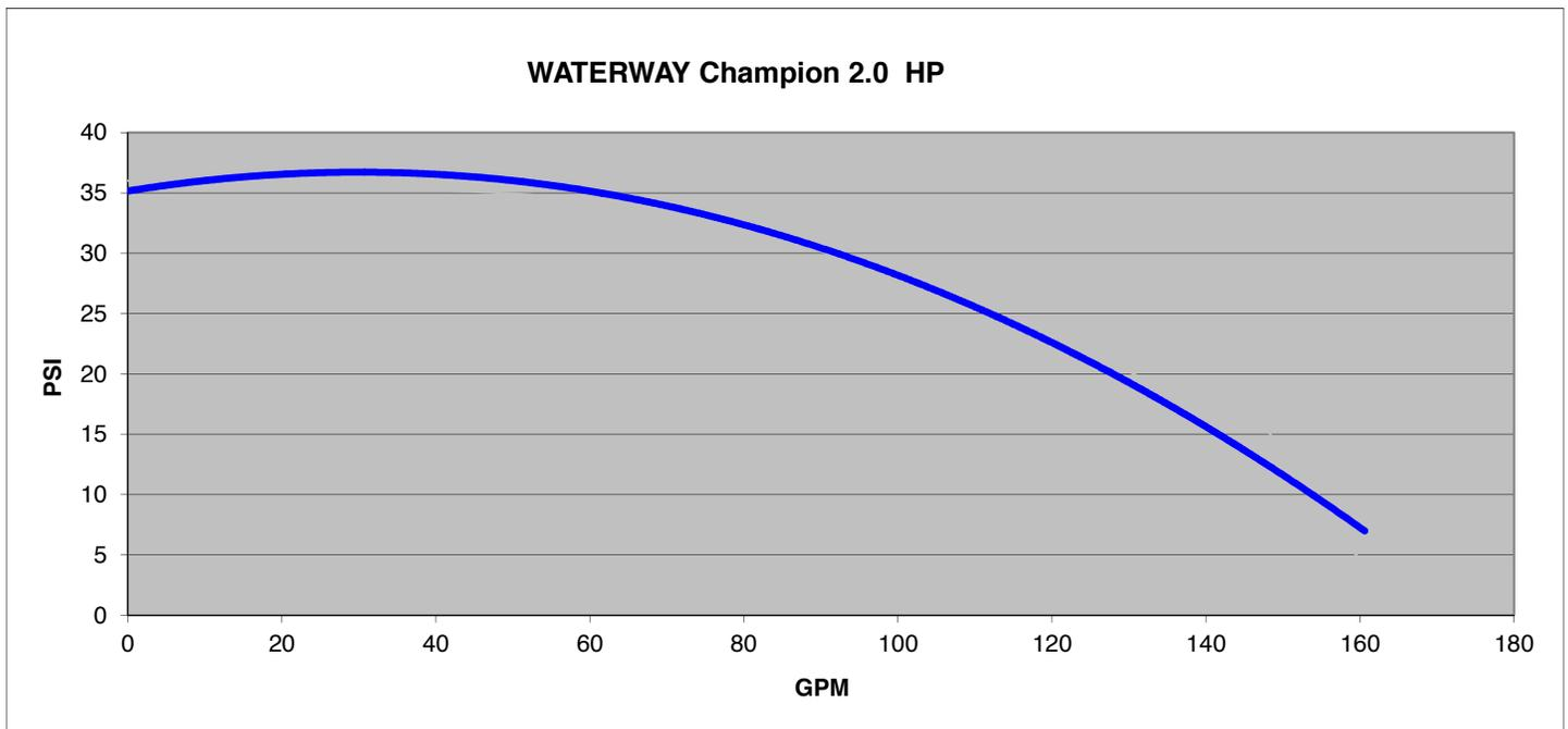
Pump curve supplied for installers where recommended pump is used.
