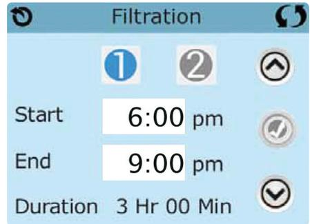
Press "1" to view Filter 1. Press "2" once to view Filter 2. Press "2" again to turn Filter 2 ON or OFF. When Filter Cycle 2 is ON, it can be adjusted in the same manner as Filter Cycle 1.
