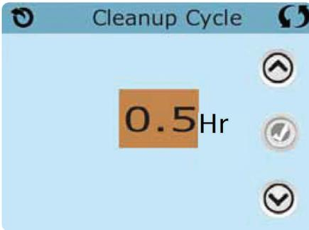
Note: Cleanup cycles do not apply to systems set for 24hr circulation pump mode as the circulation pump performs as the heat and filter pump to provide constant filtration.
