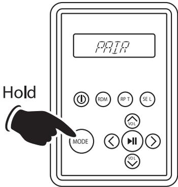
1. To pair the wireless remote with the dock push and hold the **MODE** button on the remote controller until "PAIR" appears in its display
