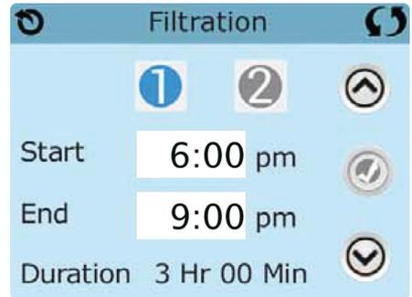
Press "1" to view Filter 1. Press "2" once to view Filter 2. Press "2" again to turn Filter 2 ON or OFF.
