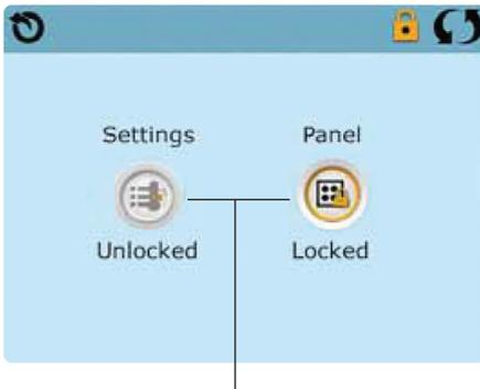
*Press and hold the Settings or Panel icon for 5-10 seconds to lock or unlock.*
