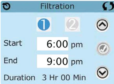
Viewing Filter 1 while Filter 2 is ON:
