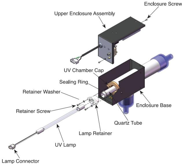
**Figure 2: Spa Solar Eclipse Exploded View**
