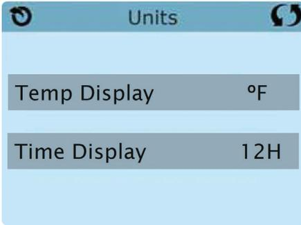
Press "Temp Display" to change the temperature between Fahrenheit and Celsius.
