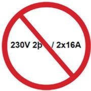
**Optional 1:** 3-Phase Service, TN and TT Electrical Systems 5 Wires (3 Lines + 1 Neutral + 1 Protective Earth)\*. Protective Earth wire (Green/Yellow) must be connected to system ground terminal as marked.
